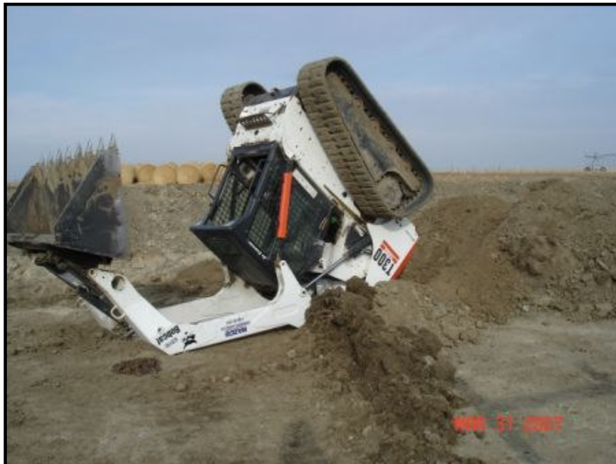
Picture #1 – Skid Steer Rollover
