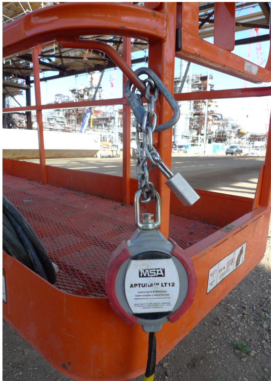
Incorrect anchorage connection
