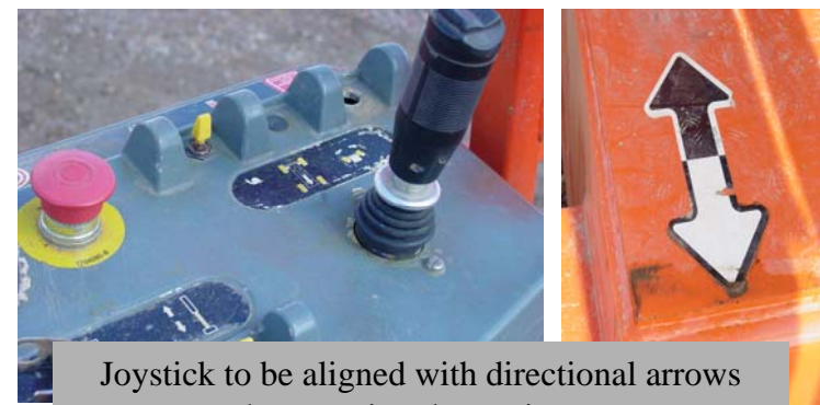
Human Factors trap when turret is rotated 180 degrees
